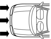
wrong with the system. Rather, it means the forces were not of the type sufficient to cause activation. Front airbags are designed to activate in frontal and near-frontal collisions, not rollover, side-impact, or rear-impacts unless the collision causes sufficient longitudinal deceleration.
